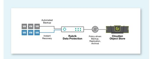
Cloudian serves as an on-premises backup, replication, and archival target for Rubrik backup processes. Policy-based tiering to the public cloud provides capacity expansion and offsite storage for disaster recovery.
