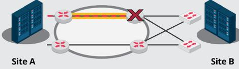
**Traditional IPsec** requires encrypted traffic be routed from a specific device to another specific device.
