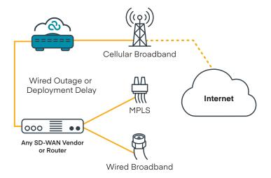
A quick and easy way to reduce the risk of a branch disconnect is to add another WAN connection. A second wire is susceptible to the same risks as the first one, and the wait for installation may be lengthy. Adding a wireless link provides both backup and diversity to the network. Rapid failover seamlessly switches from one link to another, minimizing network and service disruption.
