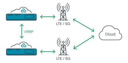
As shown, up to four carriers could be connected with dual-modem routers. Cradlepoint routers can also mirror already installed VRRP-capable routers.
