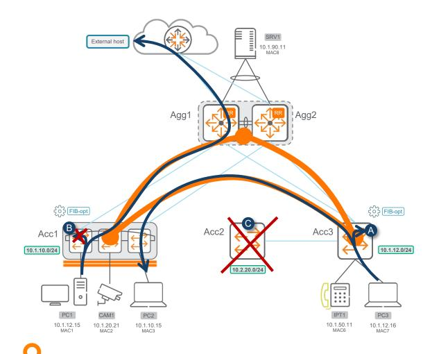
A. For each flow initiation to an EVPN host destination, a **copy of the packet** is send to the switch CPU <u>until the host route entry is programmed in HW</u>.
