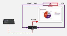
The CB Pro switches automatically to BYOM mode when detecting a connection via the button or the app. Only works with compute based room set-ups.
