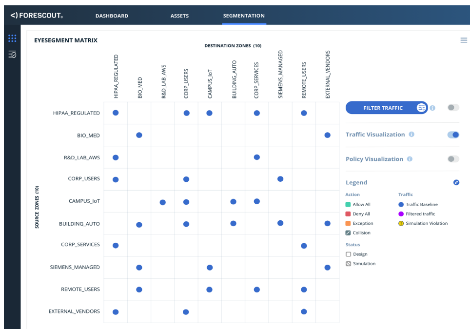
Figure 2: eyeSegment connectivity matrix view showing logical business traffic flows.
